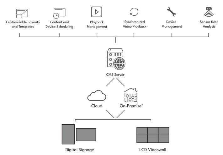
VSign is based-on three main structures which are content management, device management and sensor monitoring. The contents can be created in CMS server and sent to the displays remotely. With device management features, all Vestel displays can be controlled through Cloud or On-Premise servers. In case Vestel's Sensor Box is used with the displays, temperature, humidity, ambient light, estimated carbon dioxide, and air quality levels of the environment can be displayed in CMS server.
